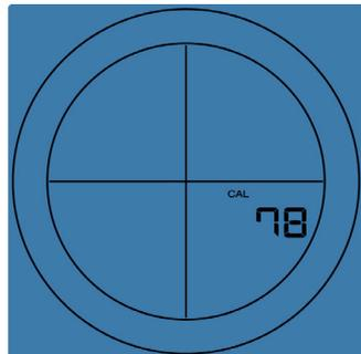
Shows the energy consumption based on a efficiency of 22% to provide the mechanical power (0-9990Kcal in 10Kcal steps).
