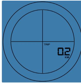
Records the distance in 0.1 km increments (0 -999.0 km). the distance is a theoretical value, which cannot be compared with the real distance on the street.
